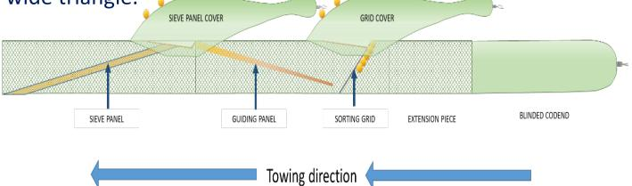
The fish and shrimp escaping from the escape openings of the sieve panel and sorting grid were collected by covers with small mesh size and codend was blinded with similar mesh size
